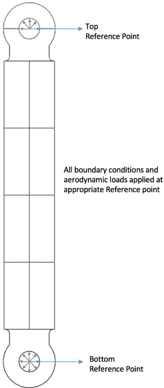
**Fig. 3. Pitch link model with rigid body tie**
