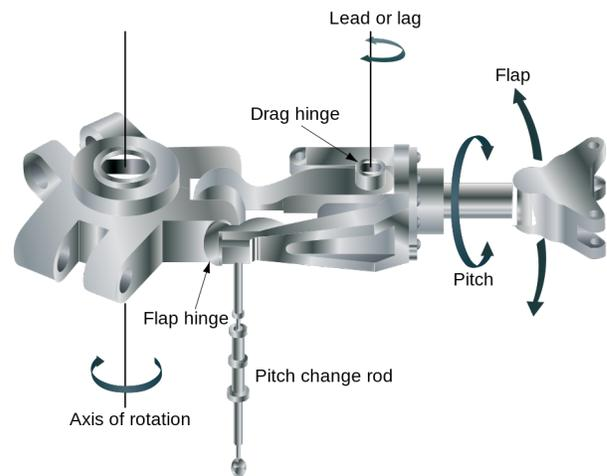
Fig. 2. Parts of fully articulated main rotor head of helicopter and the associated motions of the blades
